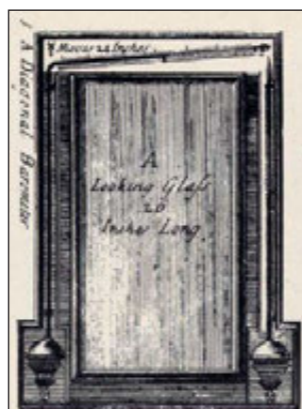
John Patrick's second advertisement, circa 1710, illustrating a 'sign-post' barometer with looking glass to centre (Banks Collection, British Museum)
